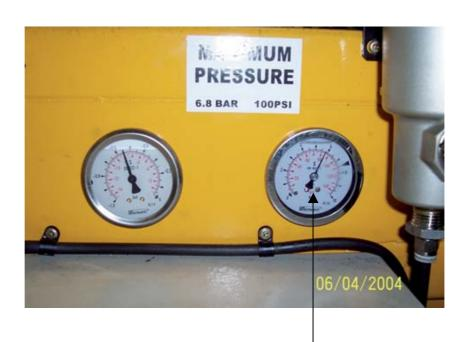
Check that pressure is positive immediately after start and rises quickly to operating pressure not to be greater than 6.3 bar or 100 psi
