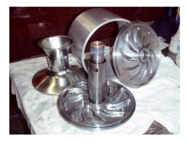
• Clean all sludge from all of the surfaces inside the rotor remembering to examine the sludge for abnormal particles.
