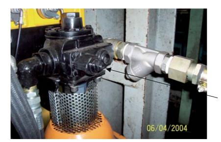
Relief Valve adjusting Screw
